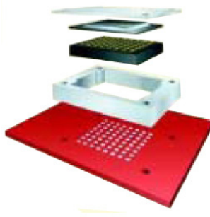
FIGURE 9: SAMTEC, WHICH PRODUCES CONNECTORS THAT TERMINATE LAND GRID ARRAY DEVICES (LGAS) TO A PRINTED CIRCUIT BOARD, USED SOLIDWORKS SIMULATION NONLINEAR ANALYSIS CAPABILITIES TO REDUCE PRESSURE AND DEFLECTION ON THE BOARD TO ACCOMMODATE A HIGH CONCENTRATION OF CONNECTIONS (600) IN A VERY SMALL AREA (ONE SQUARE INCH).
